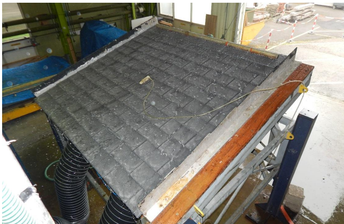
Figure 3 Tapco Classic Slates under test
