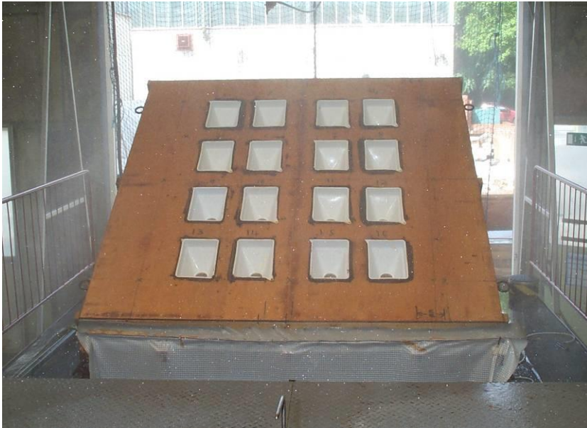
Figure B6 View of the 16 rainfall collection buckets on the test rig
