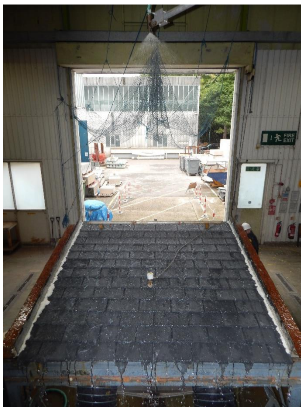
Figure 3. Tapco Classic Slate undergoing deluge testing.
