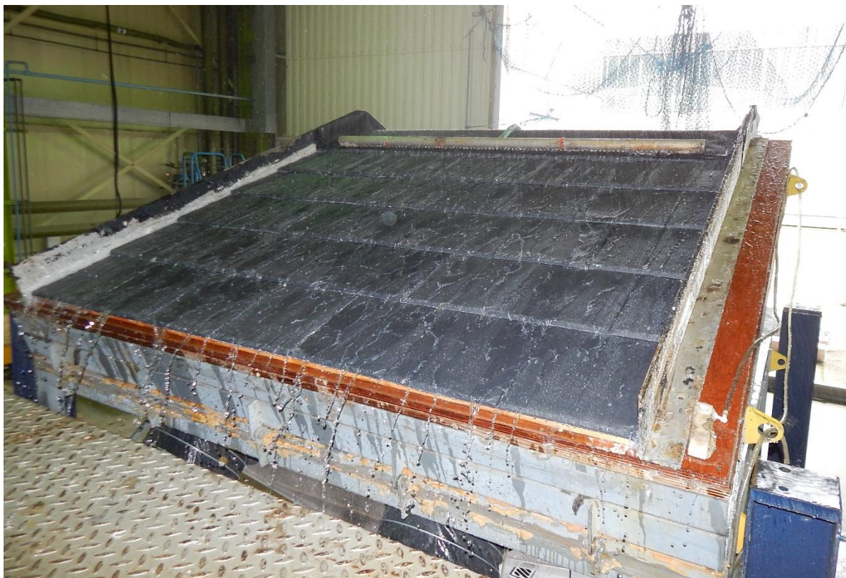
Figure 5 View of the Davinci Slates during testing
