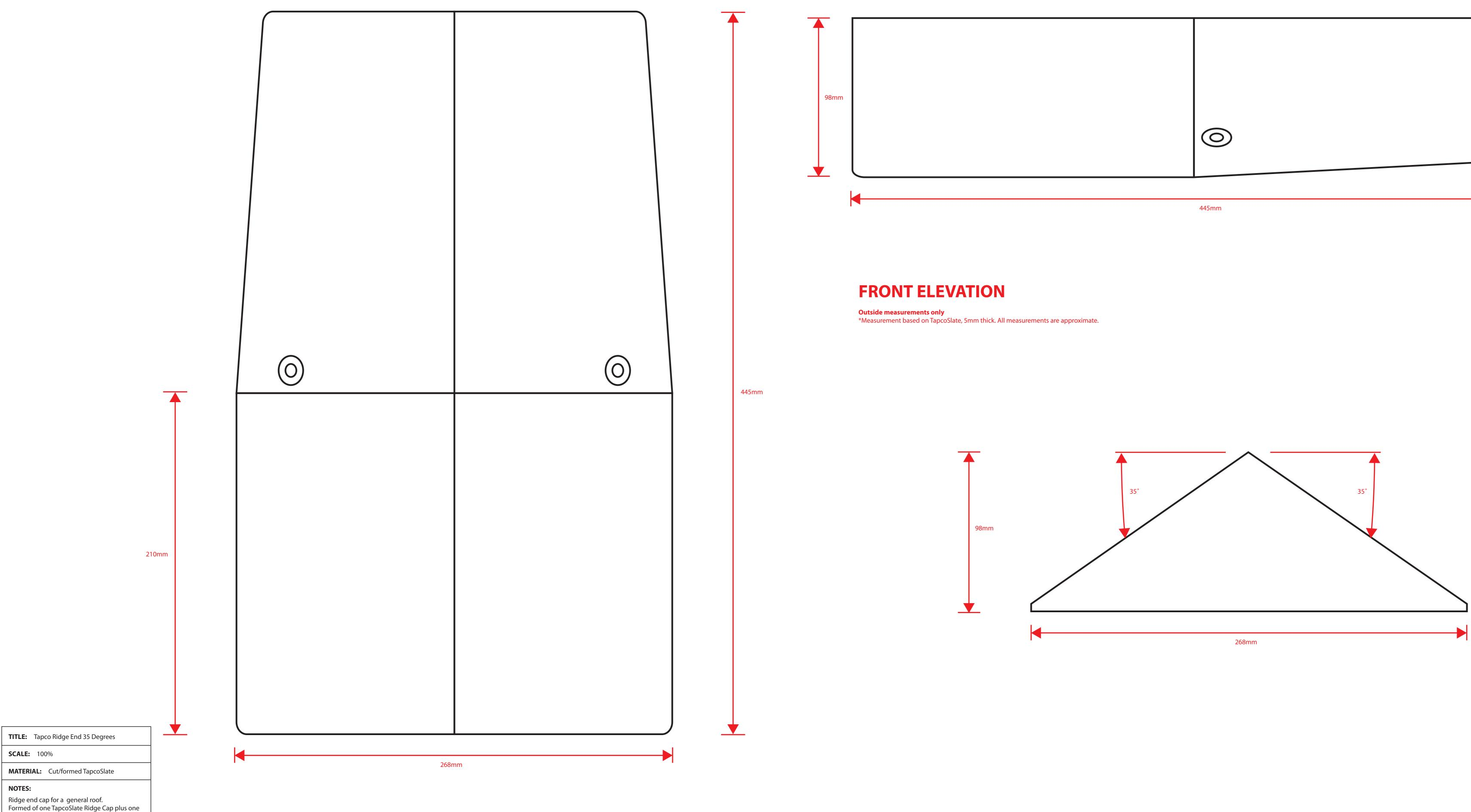
Ridge end cap for a general roof. Formed of one TapcoSlate Ridge Cap plus one TapcoSlate Tile mitred and bonded together at a 90 degree angle for the Tile and Ridge Cap set at a 35 degree angle on both sides.
