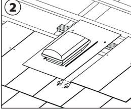
NOTE: Ensure the ventilator is not directly above a rafter and the batten cantilever is not excessive. Cut the underlay with two diagonal cuts as shown, fold back to ensure a free airpath for the ventilator, fit underlay protector (as diagram 1).
