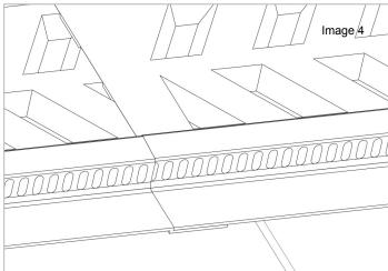
4. Moving left to right, fit the subsequent Abutment Vent by butting it to the fitted vent and repeating the fitting sequence until the full top abutment of the roof is completed. The last Abutment Vent will most likely need to be cut to ensure it finishes flush with the edge of the tiles.
