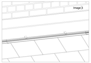
3. Ensure the slate/tiles are free from dust and remove the protection strip from the butyl strip to the underside of the front edge of the Abutment Vent and adhere the front edge to the slate/tile.
