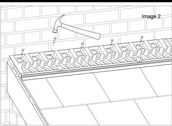
2. Starting at the end of the roof, position the first Abutment Vent so its edge is level with the edge of the tile. Ensure the vent is parallel to the wall and the front edge of the Abutment Vent sits on the tile/slates and will accommodate the flashing illustrated in 'Image 1' shown left. Fix the Abutment Vent in place as shown using 30mm galvanised round head nails.
