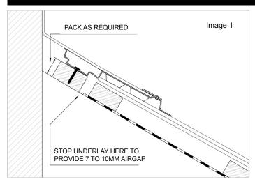
1. Prior to installation, check a suitable air gap and supporting batten for the Abutment Vent is present between the top course of tiles and wall. Depending on the tile type, additional packing may be required to support and secure the Abutment Vent.
